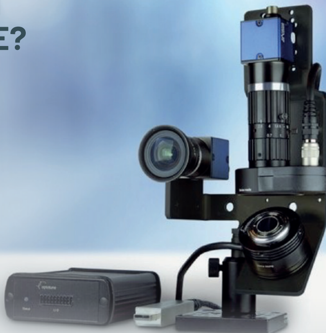
▲ Optotune's Gigapixel imaging kit comprises a wide-angle camera (left) and a narrow-angle camera (right, looking down at the mirror), which uses the liquid lens EL-16-40 for focusing and the fast-steering mirror MR-15-30 to expand the field of view to 100°.
