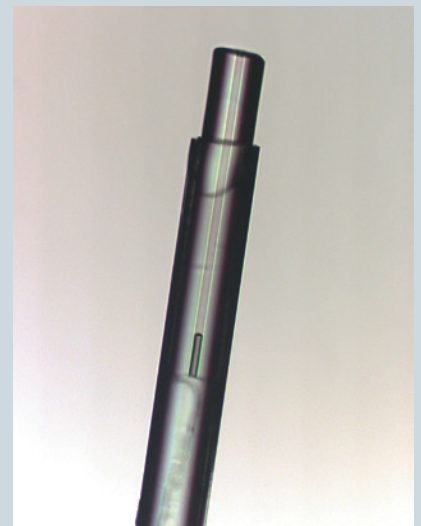
Fiber optic pressure sensor based on a tip-Fabry-Perot interferometer.
