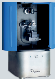
Fig. 3 Phelos analyzes angle and polarization dependent electro- and photoluminescence spectra of OLED devices and emitter films.
