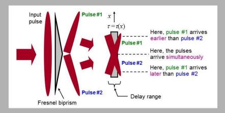
This achieves the entire range of delays for a single pulse and so yields an alignment-free single-shot measurement of a pulse.
