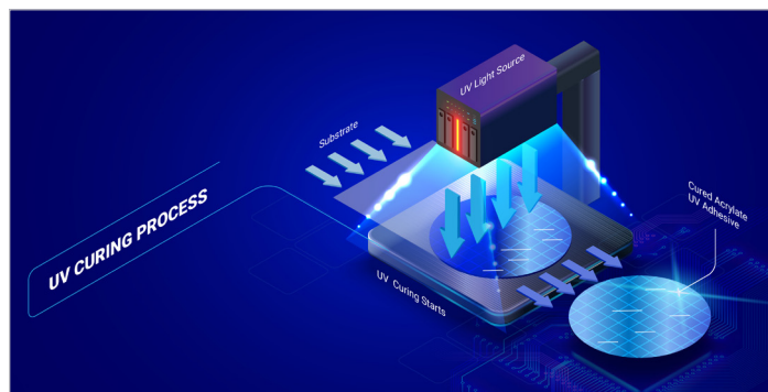
Figure 1. The use of UV curing technology is among several die-attach options commonly used in semiconductor production.
