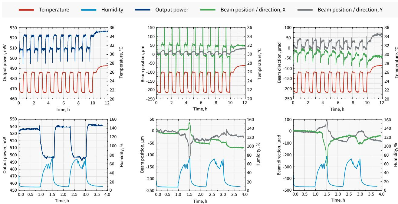
I-OFA-FW output power, beam position, and beam direction under harsh environmental conditions
