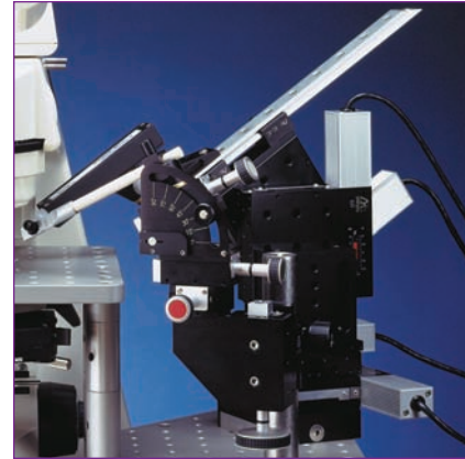
Vertical or angular platforms allow positioning of a micromanipulator at heights or angles particular to any requirement.
