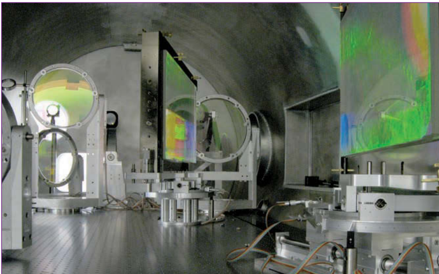
Examples of custom lens positioner mounts made for the University of Texas at Austin. The equipment is installed on a large vacuum compatible isolation table (supplied by TMC) that is inside the vacuum chamber (1x10 -6 Torr) for the university's Peta-watt laser. Photo courtesy UT-Austin
