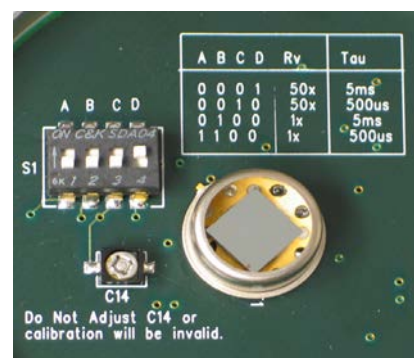
Figure 1: DIP Switch positions as indicated on the PC Board of a -BNC detector
