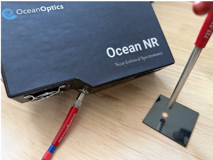
Picture 2: Reflection probe analyzing perovskite plate
