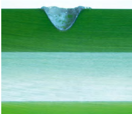
Successfully tested with a 16-kW disc laser
