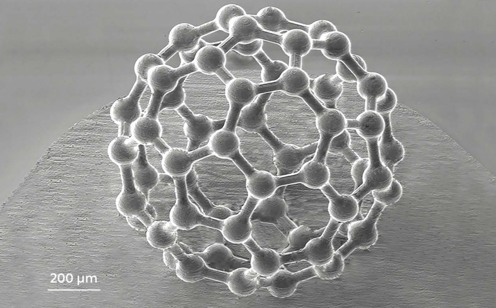
Selective laser etching is a two-step process. First, the volume of fused silica is modified by ultrashort radiation, then the material is chemically etched away. In this way, mechanically stable and durable 3D structures can be created of glass or in the volume of glass.
