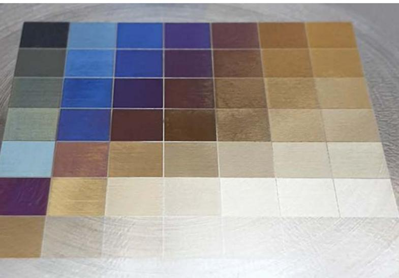
The femtosecond laser produces an oxidation formation on a titanium alloy surface. Varying colors can be achieved by creating oxide layers of different thicknesses. Electrolysis is another technology for metal coloring, but due to the precision of the laser we can selectively color the titanium with high speed and accuracy.
