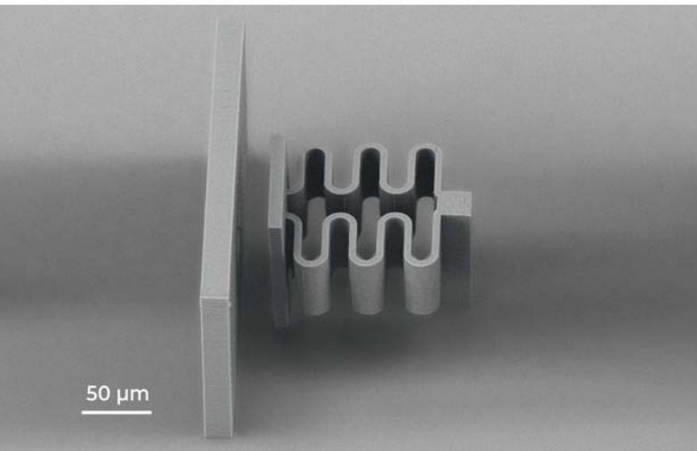
Femtosecond direct laser writing processes enable hybrid microfabrication of additive and subtractive technologies to create integrated systems. By selective laser etching (SLE), glass microstructures can be made and polymeric structures can be integrated into the glass microstructures using multiphoton polymerization (MPP).
