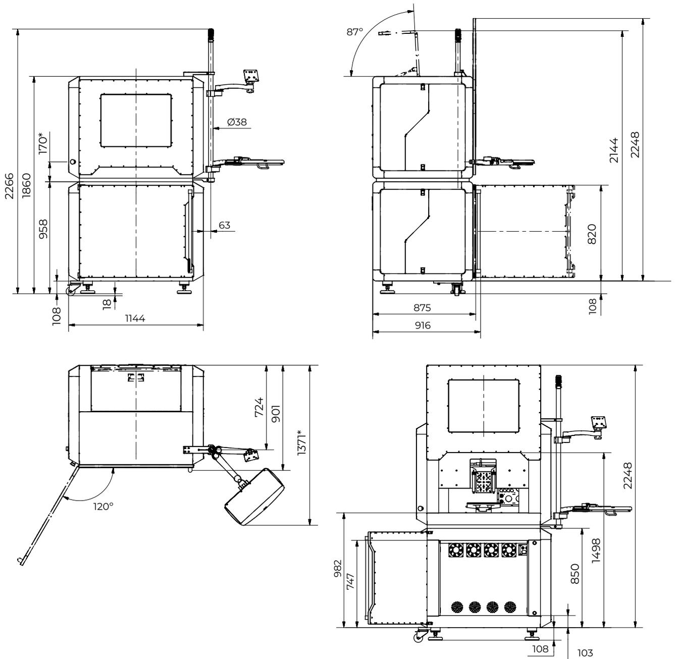
Figure 1. Laser Nanofactory dimensions in millimeters
