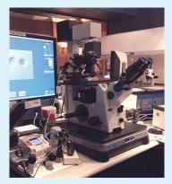
**Superior low frequency performance.** Starts to isolate at 0.7 Hz. Dramatic vibration cancellation, especially in the critical 1-10 Hz range.
