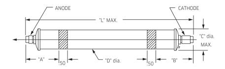
The beam exits from the anode mirror on all tubes except the 1018, 098-2 and 098-3.
