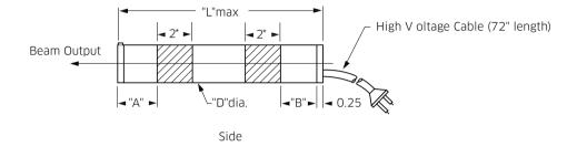
Accessory Housing Holes: M-3 on 1.38" (34.9 mm) bolt circle. (1.740" diameter head only)
