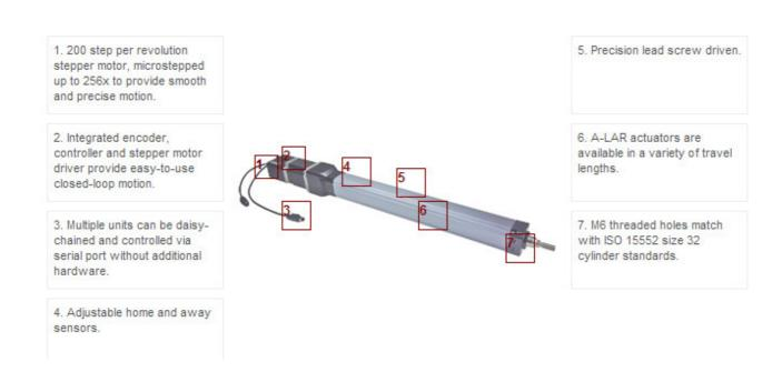
To control actuator position, simply transmit on the RS-232 port the unit number of the actuator you want to move, a simple move command and the position desired. After the move, the actuator will report its position through the RS-232 link. For a detailed list of available commands see the **A-LAR-E User's Manual**.
