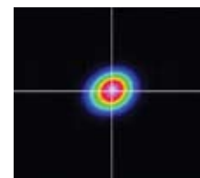
Far field from profile stable resonator at 100Hz.
