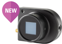
Beamage-4M-FOCUS (4.2 MPixels with 12 μm Effective Pixels 20.5 x 20.5 mm Effective Aperture)
