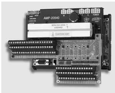
ICM-20500 Interconnect Module attached to AMP-20540 Amplifier
