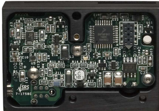
SR475 Shutter Head with cover removed, revealing control system electronics
