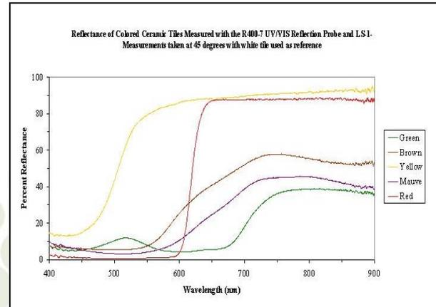
Figure 2: Reflectance of colored tiles obtained at 45 degrees
