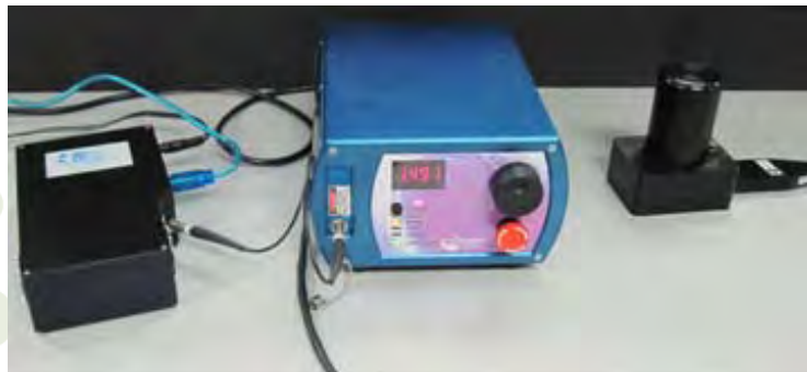
Figure 4. Equipment set-up: 785- laser, QE65000, and probe
