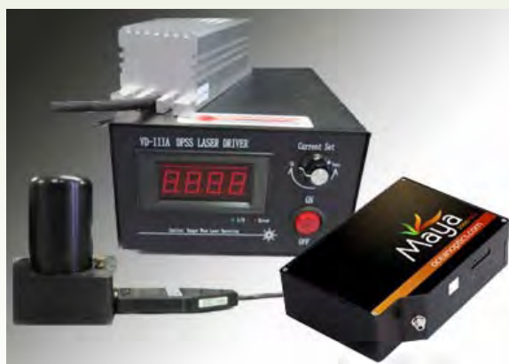
Figure 3. Equipment set-up: 532-laser, Maya2000 Pro, and probe
