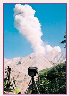
At the Montserrat Volcano Observatory (www.mvo.ms) sampling sites, spectra are collected every 4-6 seconds and transmitted to researchers at the observatory via modem; one complete scan of the plume takes 4-6 minutes. Depending on wind direction, data from two of the three spectrometers is used to calculate plume height, by comparing the angles at which peaks in the SO<sub>2</sub> plume are measured.
