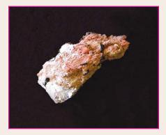
Spectrometer integration times were set for 1000 ms to measure the dim (although visible to the naked eye) genthelvite fluorescence, compared with a 10 ms integration to measure the brighter willemite fluorescence.
