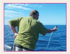
A USB4000 Spectrometer set from 360-1100 nm measures reflectance and irradiance. The USB4000 connects to a patch cord that screws into a Gershun Tube, which has fixtures for adjusting the area of light entering the fiber -- in this case, to reduce the field of view to 3°. Upwelling irradiance and downwelling radiance measurements -- the spectral distribution of the underwater light field -add valuable data.
