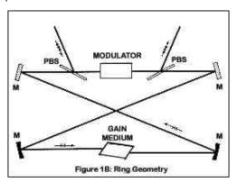
The temporial pump profile of the gain medium is considered to be CW if appreciable gain exists in the cavity for an appreciable time before the pulse to be amplified is injected and begins to increase immediately after the amplified pulse is extracted. Conoptics offers drivers for both CW pumped and non-CW pumped amplifiers.
