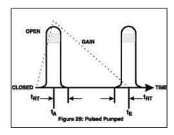
Figure 2: Driver Waveforms (not to scale)
