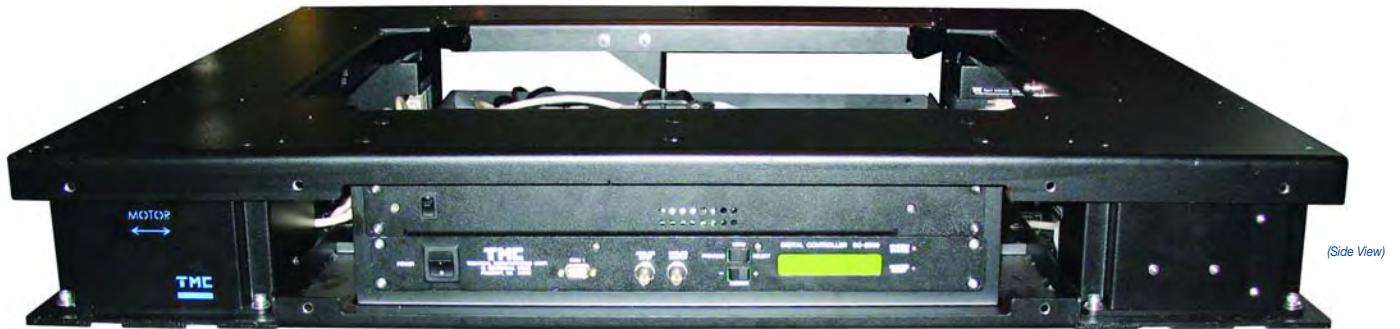
Sub-Hz Vibration Cancellation in an Active Hard-Mount Floor Platform
