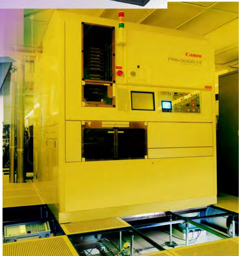
A Canon® Stepper is isolated by a STACIS® version of a TMC Quiet Island® Floor Platform.
