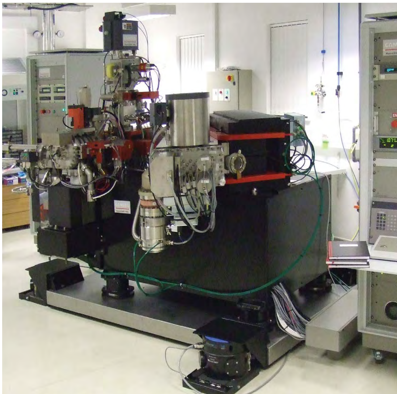
A Cameca NanoSIMS 50L on a TMC Floor Platform supported by Stacis® isolators. This tool is a 5,000-pound secondary ion mass spectrometer with a spatial resolution of 50 nanometers. Photo courtesy of the Planetary and Space Sciences Research Institute (PSSRI) at The Open University, Milton Keynes, U.K.
