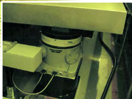
STACIS® installation at Texas Instrument's KFAB (Kilby Center), TI's most advanced research center. This Stacis platform system will be used to support and isolate an advanced metrology tool. (Pad size is 105 x 65 x 4 in. and tool weight is 6,750 lb.)
