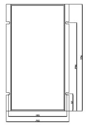
Allow 200mm clearance at rear for bend radius of umbilical. Drawings not to scale.
