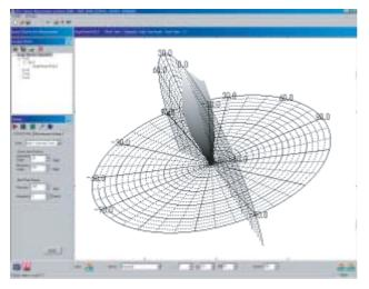
The proprietary software can show various types of graphs such as spectroradiometry, photometry, or colorimetry with 2D/3D polar/rectangular view.
