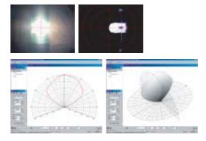
LED Profiler, IMS-5000 has released by Asahi Spectra as the most powerful instrument to evaluate unknown LED output characteristics among similar devices. The IMS-5000 can measure a spacial distribution in terms of spectral performance, illuminance, and CIE chromaticity of any illuminating object including but not limited LED. All operations are controlled by PC and the measurement is automatic.
